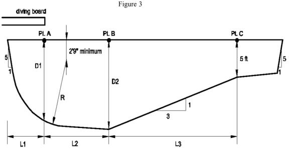
R minimum = Pool depth minus Vertical wall depth from the water line minus 3 inches.
