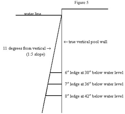
(2) The term "vertical" is interpreted to permit slopes not greater than 1 ft horizontal for each 5 ft of depth of side wall (11° from vertical).
